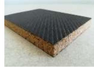
BAS630T / PFA Prepreg is a pre-impregnated basalt fabric (BAS630T) with PFA (Polyfurfuryl Alcohol) resin.
